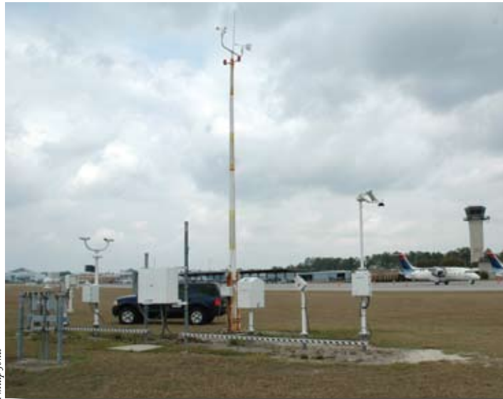
National Weather Service field instruments at Columbia Airport include present weather sensors for temperature, dewpoint, rain, freezing rain, snow and fog, wind speed and direction, visibility and ceiling.
